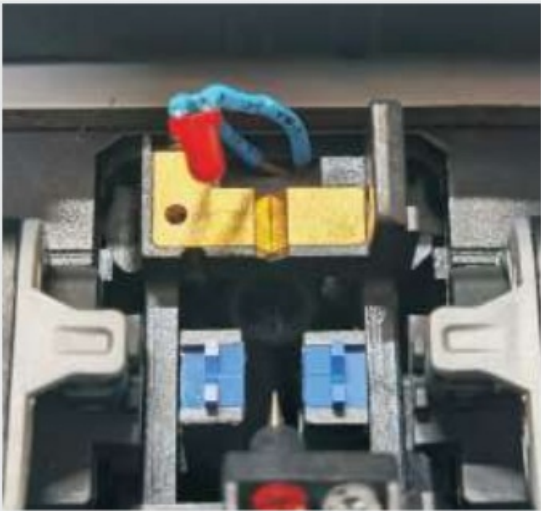
9. Replace the new electrode and put the copper gasket back to slot please note that keep the copper gasket's wide gaps towards to the tips side.
